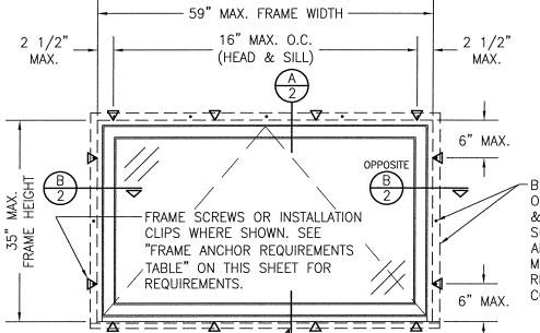
BRICK MOLD AND ANCHORING OF BRICK MOLD IS OPTIONAL & SHALL NOT ACT AS A SUBSTITUTE FOR THE FRAME ANCHORS SPECIFIED. BRICK MOLD MAY BE REMOVED WHEN REQUIRED BY OPENING CONDITIONS
