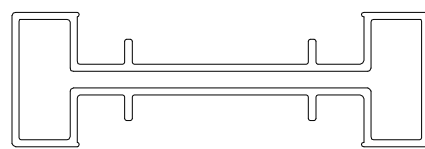
PROFINISH LARGE VINYL H-MULLION COVER #VPI-560 EXTRUDED VINYL 0.079" MIN.
