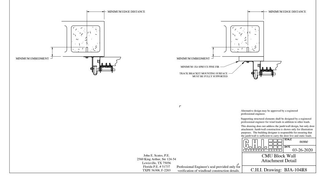
1/4" Tapcon+ (PLUS) Minimum Embedment 2.0", Minimum Edge Distance 1.63", Minimum spacing 3"
