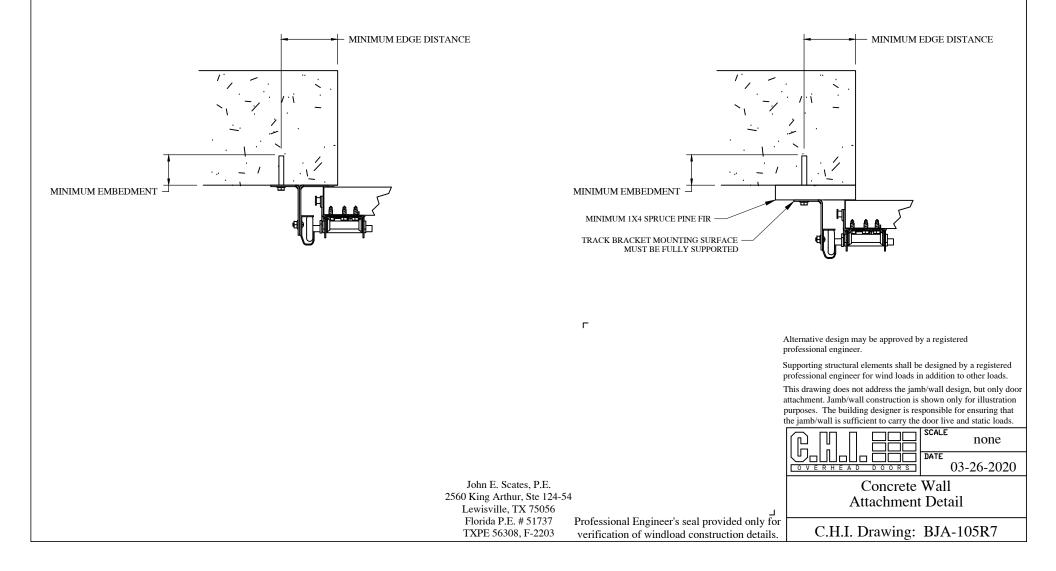
Refer to door drawing installation instructions for bracket spacing.
