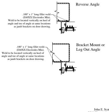
Welds performed by a Certified Welder or inspected by a Certified Welding Inspector to verify integrity of welds. 12 gauge or  $\frac{1}{5}$ 's steel Jambs; allowable load per weld= 1,272 lbs. Use all necessary precautions when welding galvanized steel. Locate welds in same location as jamb brackets on door drawing.
