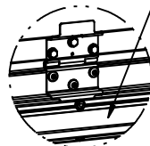
AFTER U-BAR INSTALLATION
