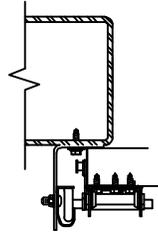
Screw: 1/4" dia x 3/4" self tapping screw; must conform to ANSI/ASME B18.2.1.
