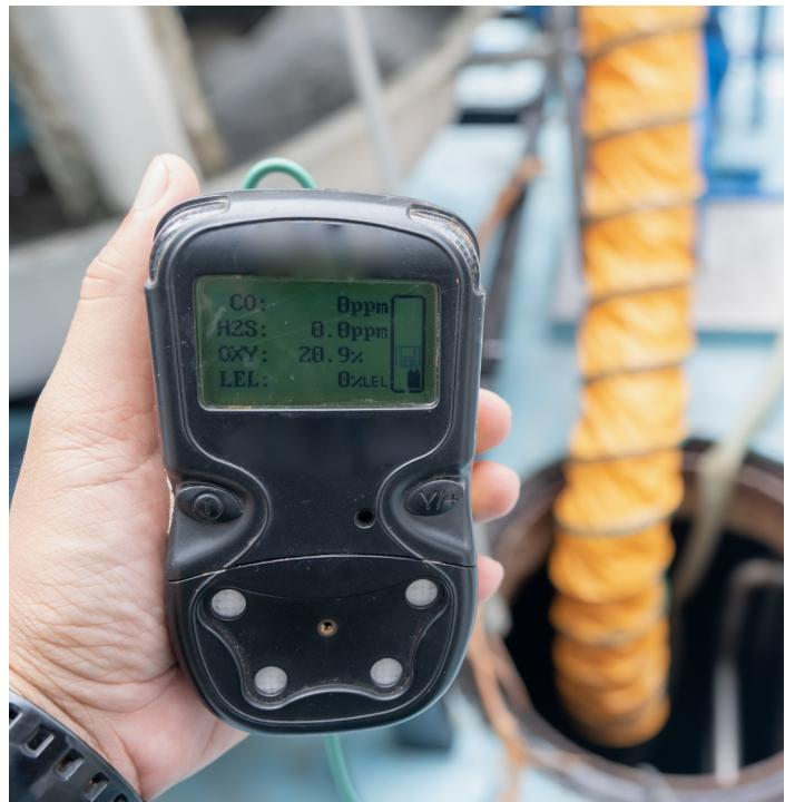
before permitting entry. If ventilation is impossible and entry is necessary, employees must wear the proper respiratory protection for the detected contaminants.
