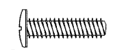
15 1/4-20 TRUSS HEAD BOLT REQUIRES USE OF KEYHOLE WASHER IN DIRECT MOUNT APPLICATIONS
