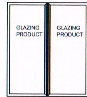
2-WAY VERTICAL MULLION CONFIGURATION
