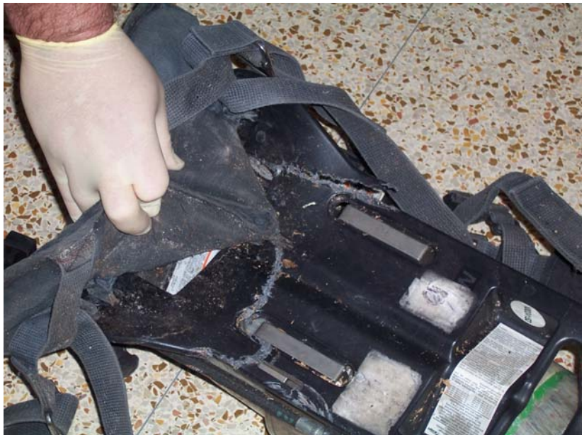
Figure 12. Photograph of the SCBA frame damage illustrating the cracked bracket (Photo by TCFP)
