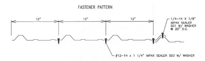
Figure 1. R-Panel PB Panel Fastening Details
