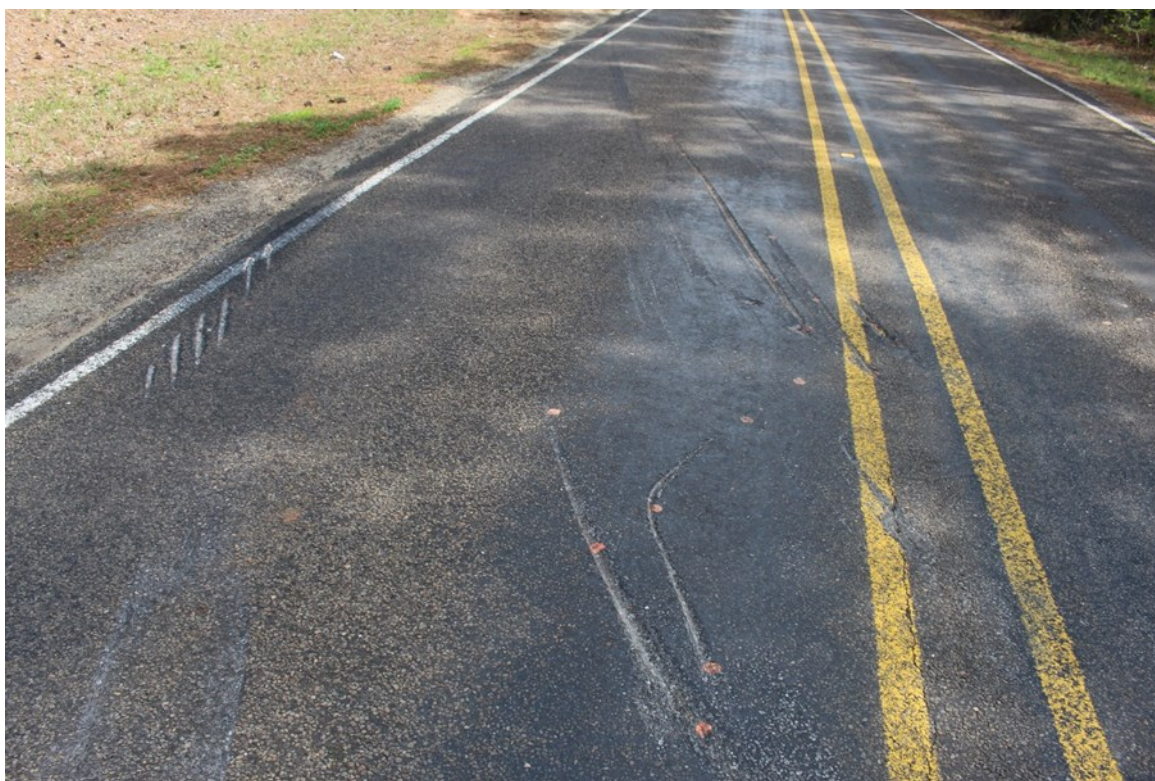
Impact marks from passenger side of the apparatus as it rolled over. ( Photograph by SFMO Lt. Brian Fine )
