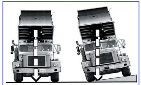
A slight slope can be enough to cause tipping if material sticks in the top of the box.
