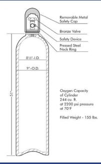
Compressed Gas Hazards Compressed gas cylinders come in different shapes and designs, which are mostly based on the pressure of the gas they contain. In general, they are grouped as high-pressure cylinders, low-pressure cylinders, and cryogenic containers.<sup>5</sup>
