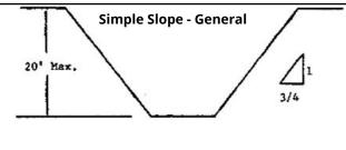
Exception: Simple slope excavations which are open 24 hours or less (short term) and which are 12 feet or less in depth shall have a maximum allowable slope of ½:1.
