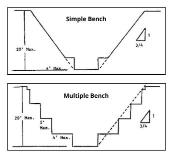
3. All excavations 8 feet or less in depth which have unsupported vertically sided lower portions shall have a maximum vertical side of 3½ feet.
