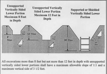
All excavations 20 feet or less in depth which have vertically sided lower portions that are supported or shielded shall have a maximum allowable slope of 3/4:1. The support or shield system must extend at least 18 inches above the top of the vertical side.
