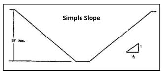
2. All excavations 20 feet or less in depth that have vertically-sided lower portions shall be shielded or supported to a height at least 18 inches above the top of the vertical side. All such excavations shall have a maximum allowable slope of 1½:1.
