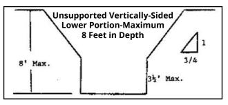
All excavations more than 8 feet but not more than 12 feet in depth with unsupported vertically sided lower portions shall have a maximum allowable slope of 1:1 and a maximum vertical side of 3½ feet.
