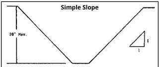
2. All benched excavations 20 feet or less in depth shall have a maximum allowable slope of 1:1 and maximum bench dimensions as follows:
