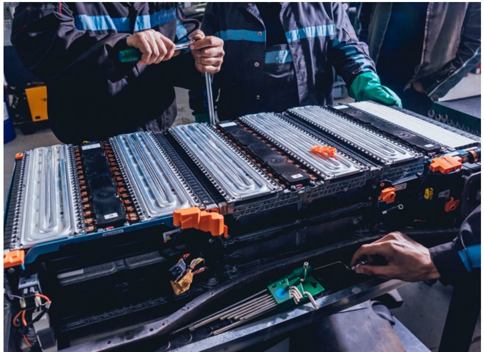
Disassembling the battery of an electric vehicle.
